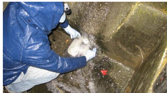
Figure 9. Collecting a sheet flow stormwater sample.
